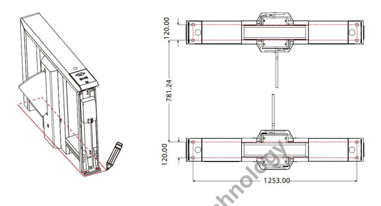
5. Take the turnstile aside and use the electric drill according to the drawn screw holes.
