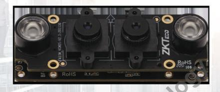
FA11M is a high-performance face capture module that combines with visible light and near-infrared cameras. It is equipped with binocular wide dynamic image sensors and an aspherical distortion-free camera and near-infrared illumination lights.
